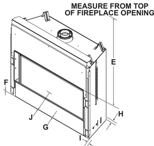
The rough framing dimensions shown represent the distance from stud to stud only and do not take into consideration the addition of drywall.
